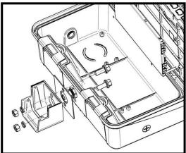
1. Install the small piece of the Universal Pole Mount Bracket oriented as Shown using the provided hardware. Gasket must be placed between the UPMB and the casting to preserve IP rating. Tighten nuts to 12 ft-lbs.
