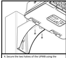
4. Secure the two halves of the UPMB using the provided #10-32 screws.
