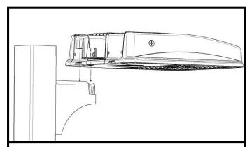
3. Slide fixture with small piece attached over the large piece, so that the cutout on the small piece aligns with the large piece. The top surfaces of both pieces should be nearly flush.
