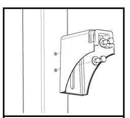
2. Install the large piece of the Universal Pole Mount Bracket to the pole using existing holes. The mounting holes and slots in the UPMB are designed for  $\aleph''$  hardware (provided by others).
