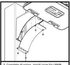
5. Complete all wiring. Install cover for UPMB using the provided #8-32 screws.
