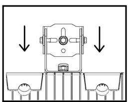
4. Screw in the top bolt/anchor until the head is about 1/4" from the mounting surface. Slide the large portion of the keyhole slot over the bolt and slide the fixture down until the bolt touches the top of the keyhole.
