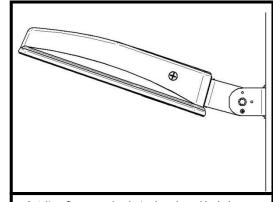
6. Adjust fixture to the desired angle and lock the bracket in place by reinstalling the #10 screw. Tighten the bolts on the sides of the bracket to 10 ft-lbs.
