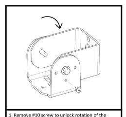
Swivel Bracket. Adjust the bracket to a 90-degree
