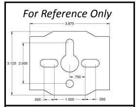
3. Reference the included drawing to mark hole locations on the intended mounting surface. Pre-drill holes as needed. AL-SB is intended to be mounted with 3/8" lag screws or concrete anchors (provided by others).
