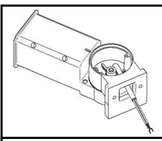
5. Set the desired angle of the slipfitter using the angle measurements on the cover for reference. Tighten the large bolt connecting the two halves of the slipfitter to 15 ft-lbs.
