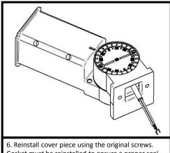
Gasket must be reinstalled to ensure a proper seal.
