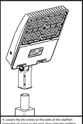
9. Loosen the (4) screws on the sides of the slipfitter. Complete all wiring to the pole, then slide the slipfitter onto the tenon. Tighten the (4) screws to 15 ft-lbs.
