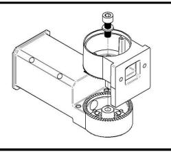
Remove the large bolt connecting the two halves of the slipfitter together. Collect and save all hardware and gaskets.
