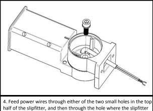
4. Feed power wires through either of the two small holes in the top half of the slipfitter, and then through the hole where the slipfitter will mount to the fixture. Reinstall the large bolt and washer to connect the two halves of the slipfitter together.
