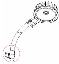
Attach the mounting clamp to the arm and secure with the provided hardware. Ensure the clamp does not rotate on the arm before continuing.
