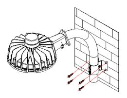
Attach luminaire and arm assembly to wall or vertical surface securely with four screws. Apply silicone sealant around wire/wall opening. Restore power to circuit and test to confirm proper operation.
