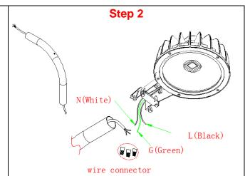
Feed supply wires through the arm assembly and connect to the power leads from the fixture. Slide the fixture over the arm and clamp securely. Ensure the fixture does not rotate on the arm before continuing.
