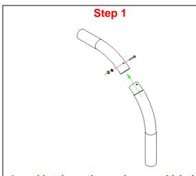
Assemble tube sections and secure with locknut (note: one section may be used to aim luminaire at high angle for longer forward light throw)
