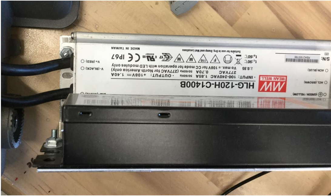
Figure 2: Attach Driver to Plate with Domed Nuts
