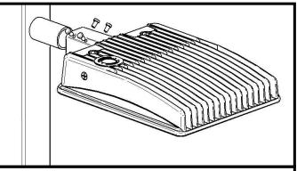
3. Feed power wires from the pole into the fixture. Loosen the four bolts on the sides of the Adaptor and slide it over the tenon. Check to ensure the fixture is level, and tighten the four bolts on the sides of the Adaptor to 15 ft-lbs. Complete all wiring inside fixture. Tighten cord lock and close the driver compartment, securing it with the latches.
