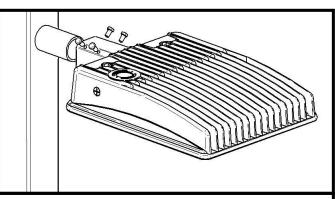
3. Feed power wires from the pole into the fixture. Loosen the four bolts on the sides of the Adaptor and slide it over the tenon. Check to ensure the fixture is level, and tighten the four bolts on the sides of the Adaptor to 15 ft-lbs. Complete all wiring inside fixture. Tighten cord lock and close the driver compartment, securing it with the latches.
