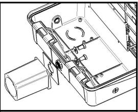
2. Install the Horizontal Tenon Mount Adaptor with the hardware provided, placing the provided gasket between the Adaptor and the fixture. Tighten both bolts to 12 ft-lbs.
