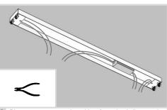
5 Disconnect or sever the wiring from the ballast to the fluorescent lamp sockets.
