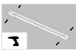
13 Fit the LED Channel around the existing fixture and attach it using at least four (4) of the provided Self-Drilling Screws. There should not be any gaps between the LED Channel and the original fixture housing.
