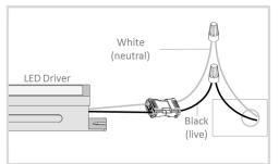
**9** Connect AC input cables to the incoming AC power connection using the proper connectors in accordance with current state and federal regulation.
