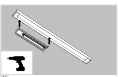
If the LED Driver comes attached to the LED Driver Plate, install the Driver Plate using the two (2) Driver Screws.
