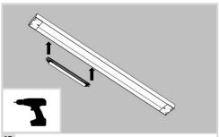
8B If there is no LED Driver Plate, install the LED Driver using the two (2) Driver Screws.
