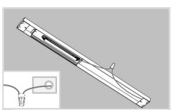
10B If the original fixture ground connection is NOT attached to the fixture housing, connect it to the ground cable (green) using the proper connectors in accordance with current state and federal regulation.
