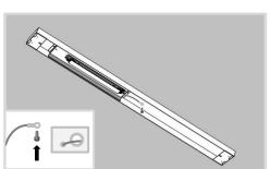
10A If the original fixture ground connection is attached to the fixture housing, use a provided self-drilling screw to attach the ground cable (green) to the fixture housing.
