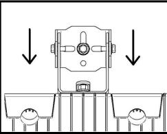
4. Screw in the top bolt/anchor until the head is about 1/4" from the mounting surface. Slide the large portion of the keyhole slot over the bolt and slide the fixture down until the bolt touches the top of the keyhole.
