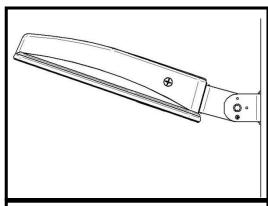
6. Adjust fixture to the desired angle and lock the bracket in place by reinstalling the #10 screw. Tighten the bolts on the sides of the bracket to 10 ft-lbs. NOTE: Max tilt 70 degrees from horizontal plane.
