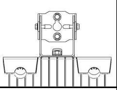
5. Install the remaining bolts/anchors, and tighten all to 18-20 ft-lbs. Complete all wiring and close and latch the driver compartment.
