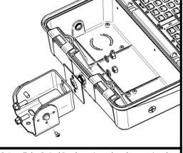
2. Install the Swivel Bracket oriented as shown using the provided hardware. Gasket must be placed between the Bracket and the casting to preserve IP rating. Tighten nuts to 12-15 ft-lbs.
