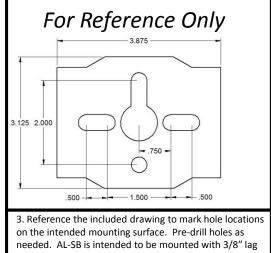
screws or concrete anchors (provided by others).
