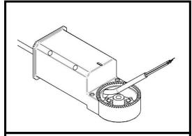
Feed power wires into the bottom of the slipfitter arm and through the hole that leads into joint of the arm.
