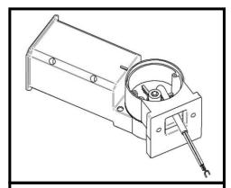
5. Set the desired angle of the slipfitter using the angle measurements on the cover for reference. Tighten the large bolt connecting the two halves of the slipfitter to 15 ft-lbs.
