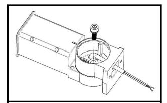
4. Feed power wires through either of the two small holes in the top half of the slipfitter, and then through the hole where the slipfitter will mount to the fixture. Reinstall the large bolt and washer to connect the two halves of the slipfitter together.
