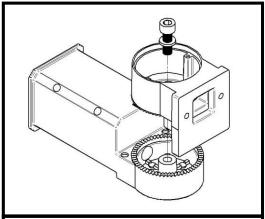
2. Remove the large bolt connecting the two halves of the slipfitter together. Collect and save all hardware and gaskets.
