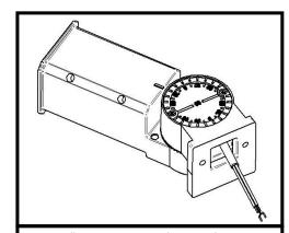
6. Reinstall cover piece using the original screws. Gasket must be reinstalled to ensure a proper seal.
