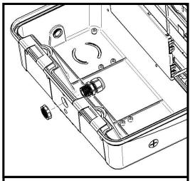
7. Reverse cord lock so that it is installed as shown, with the domed sealing nut on the inside of the fixture. Tighten lock nut to 40 in-lbs.
