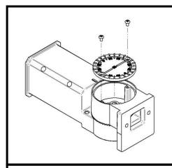
1. Remove the cover piece from the slipfitter. Collect and save all screws and gaskets to reinstall later.
