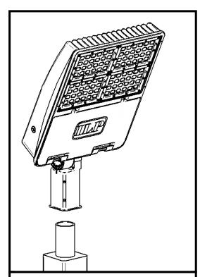
Loosen the (4) screws on the sides of the slipfitter.
