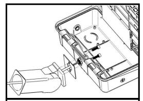
8. Feed power wires through the provided gasket pad and into the cord lock. Secure the arm to the fixture using the bolts provided. Tighten the bolts to 12-15 ft-lbs. Complete all wiring inside the fixture.
