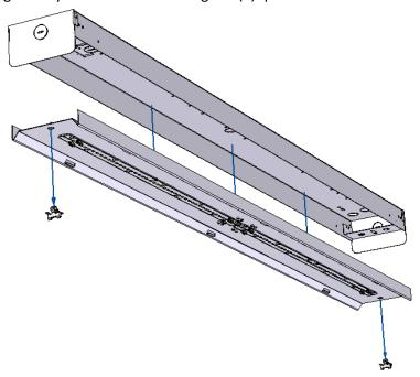
3) Place fixture against desired surface then drill through the back of the housing with suitable screws to attach the fixture to the ceiling. Make sure fixture is attached according to local and federal standards.
