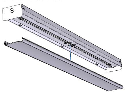
2) Remove the LED gear tray from the fixture using the (2) quarter-turns.
