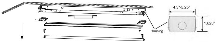
Remove ballast cover, ballast, socket-bars and wiring
