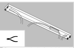
5 Disconnect or sever the wiring from the ballast to the fluorescent lamp sockets.
