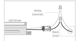
10 Connect AC input cables to the incoming AC power connection using the proper connectors in accordance with current state and federal regulation.
