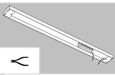
7 Disconnect or sever the wiring from the AC power input to the fluorescent ballast. If space is limited, remove the ballast.
