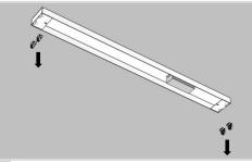
**6** Remove the fluorescent lamp sockets and any wiring that may still be attached.
