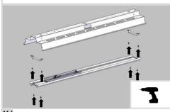
11d (LOWBAY MOUNT) Install brackets to the housing as shown using four (4) self-drilling screws. Then fit the LED gear tray assembly to the brackets to using four (4) more of the provided self-drilling screws.
