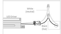
10 Connect AC input cables to the incoming AC power connection using the proper connectors in accordance with current state and federal regulation.
