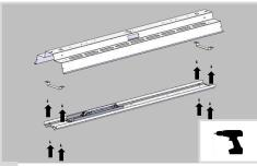
11d (LOWBAY MOUNT) Install brackets to the housing as shown using four (4) self-drilling screws. Then fit the LED gear tray assembly to the brackets to using four (4) more of the provided self-drilling screws.
