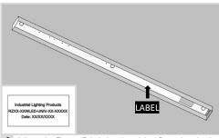
8 Adhere the Fixture ID Label to the original fixture housing in a clearly visible location. This label is required by UL standards.
