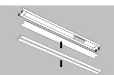
4 Remove fluorescent lamps and ballast cover. Dispose of the lamps in proper accordance with current state and federal regulation. Fluorescent lamps contain hazardous materials.
