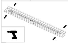
11a (FIXED WIDTH STRIP MOUNT) Fit the LED Channel around the existing fixture and attach it using at least four (4) of the provided self-drilling Screws. There should not be any gaps between the LED gear tray assembly and the original fixture
