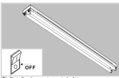
3 Shut off or disconnect power to the fixture.
