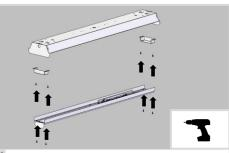
(SURFACE MOUNT) Install brackets to the housing as shown using four (4) self-drilling screws. Then fit the LED gear tray assembly to the brackets using at least four (4) more of the provided self-D\drilling Screws.
