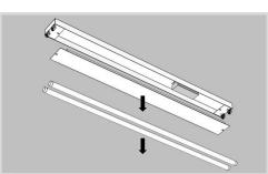
4 Remove fluorescent lamps and ballast cover. Dispose of the lamps in proper accordance with current state and federal regulation. Fluorescent lamps contain hazardous materials.
