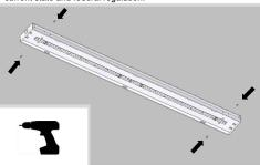
11a (FIXED WIDTH STRIP MOUNT) Fit the LED Channel around the existing fixture and attach it using at least four (4) of the provided self-drilling Screws. There should not be any gaps between the LED gear tray assembly and the original fixture housing.
