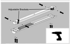
11b (ADJUSTABLE STRIP MOUNT) Fit the adjustable brackets as shown and bend them to wrap around the housing. Secure the brackets to the housing with four (4) self-drilling screws. Then fit the LED gear tray assembly to the brackets using at least four (4) of the provided Self-Drilling Screws.
