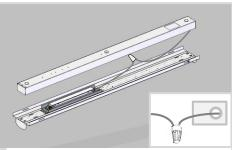
9 Ground the fixture using the ground cable (green) with proper connectors in accordance with current codes and regulations.
